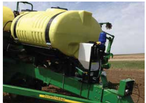
Typical mounting of 19-gallon INDEX holding tank and Dosatron system on planter.
