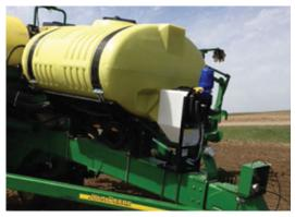
Typical mounting of 19-gallon **INDEX** holding tank and Dosatron system on planter.
