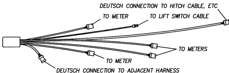
Figure 13 - 4-Row Wiring Harness
