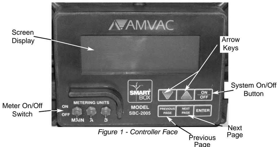
Figure 1 - Controller Face
