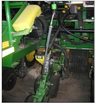
MID; PVC LONG approximately <sup>3</sup>/<sub>4</sub>" from the end. Place this marked end up into the SLIDE TUBE, BONDED LONG.
