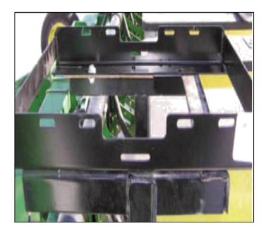
C. The SmartBox<sup>®</sup> base container (with meter installed on base container) can now be installed.
