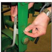
**General Mounting Instructions**: Your SmartBox® system requires that a minimum 45 degree angle be maintained at any point along the product discharge path from the meter outlet to the in-furrow drop tube. The drop tube may need to be bent to adjust. The plastic hose should be cut to length to eliminate any unnecessary slack that could cause a flow restriction. Also, if using a seed firmer the drop tube's foot (if applicable) may need to be cut off or bent up if restricting the firmer's travel.
