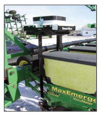
A. First, locate the four holes for mounting, and then remove the bolts mounting the down pressure springs (if equipped). Using the bushings and new hardware provided, re-attach the down pressure spring (if equipped) and the mounting bracket to the parallel arms, making sure to have the mounting brackets open section (top) facing forward toward the front of the planter. Tighten all four bolts so the bracket is secure to the row unit.
