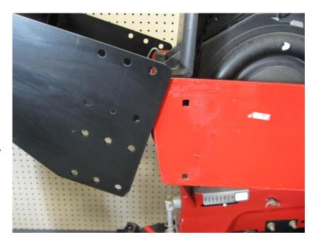
C. Fasten both sides of bracket using the four (4) bolts, washers and locknuts (*item no. 2, 3 and 4*) provided.
