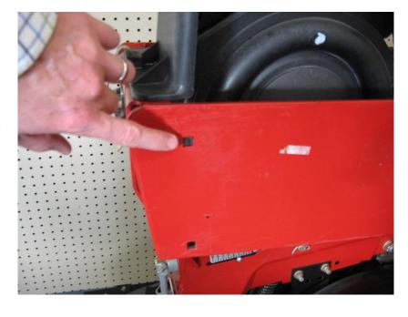
B. Slide the bracket over the side panels of the row unit and align the holes.
