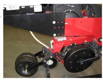
A. The bracket will mount to the row unit's side panels using the existing holes.
