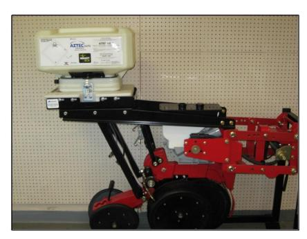
A. Remove the nuts and bolts that fasten the top parallel arm links to the row unit.
