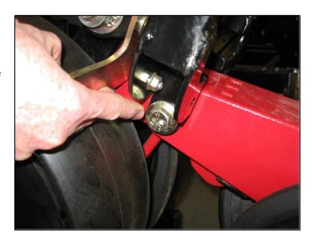
C. Fit the Plate; SB, Base (item no. 11) over the left and right Angle Plates and Tube Braces. Align all three (3) Base Plates bolt holes with the three (3) bolt holes of the Angle Plates. The Tube Braces will be aligned with the center holes of the left and right Angle Plates. Fasten using bolts and locknuts (item no. 3 and 7).
