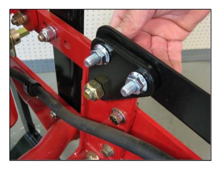
B. Remove the row unit's closing wheel assembly pivot bolt on one side of the planter.
