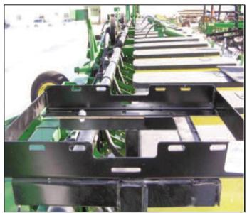
E. The SmartBox<sup>®</sup> base container (with meter installed on base container) can now be installed.
