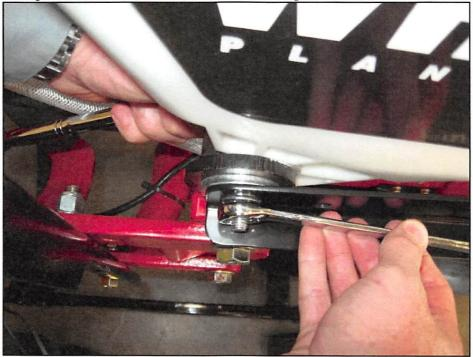
B. Remove the row unit's closing wheel assembly's pivot bolt on one side of the planter. Use this same bolt to install Item No. 15 (WELDMENT; TUBE BRACE). Repeat this process on the opposite side of the row unit.
