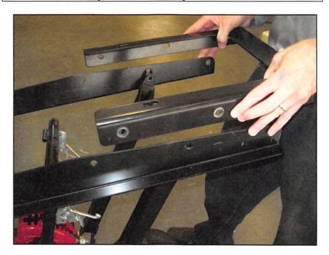
D. The SmartBox Cradle will be then hooked into the rear of the Base Plate and secured with four bolts and locknuts provided with the SmartBox Row Unit's hardware. Refer to the AMVAC SmartBox System Parts and Operator's Manual regarding the installation of the remainder of the system.
