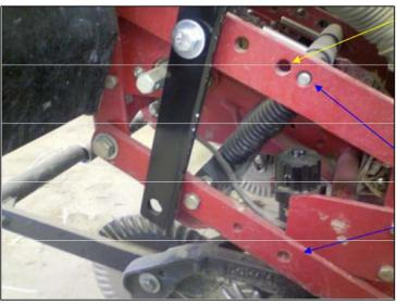
B. Using the bushings and new hardware provided, attach the mounting bracket to the parallel arms in the last rear holes, making sure to have the mounting brackets open section (top) facing forward toward the front of the planter. Tighten all four bolts so the bracket is secured to the row unit.
