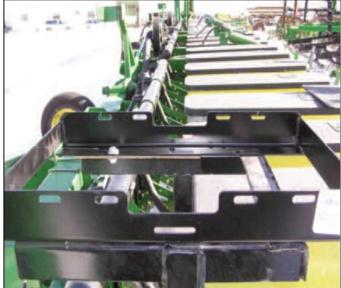
D. The SmartBox<sup>®</sup> base container (with meter installed on base container) can now be installed.
